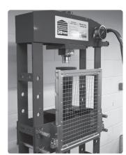
4.2. Take the guard and slide it into the brackets from above; the guard has a stop on either side at the top of the frame, this should be uppermost and facing towards the operator fig.3.
